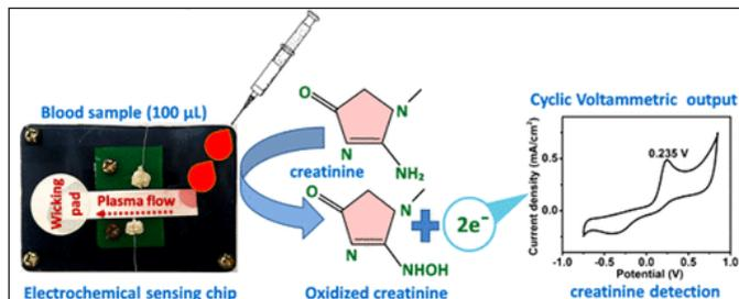
Fig 4: Schematic diagram of reduced graphene oxide based creatinine detection (Reproduced with permission from ref. 11. Copyright (2021) American Chemical Society)
